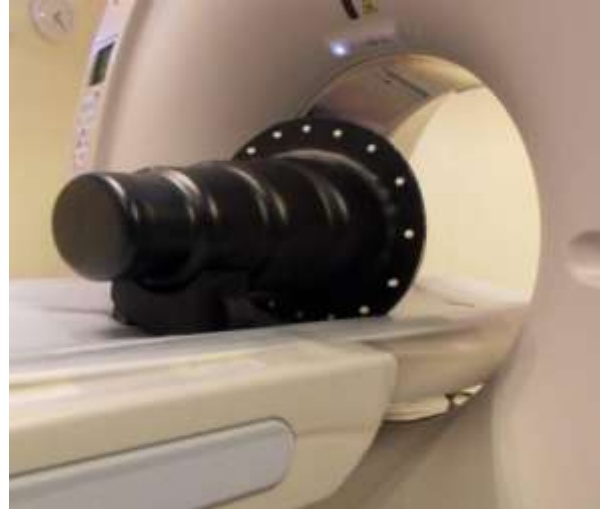
BOD phantom and CeLT phantom (North Wales Medical Physics)
