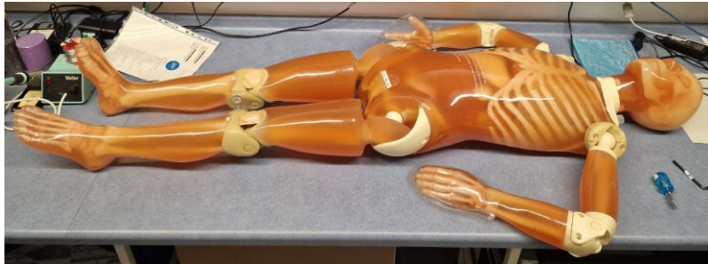
PBU-60 Whole Body Phantom 165 cm, 50 kg → BMI 18.4 (packing weight 80 kg)
